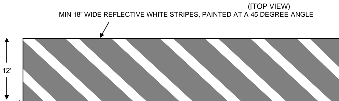
DIAGRAM A-3.5: SPEED HUMP STRIPING
